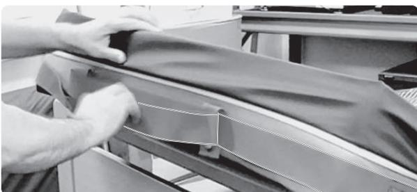
8. Pull the drag straps away for the retaining tabs to extend the drag strap.
