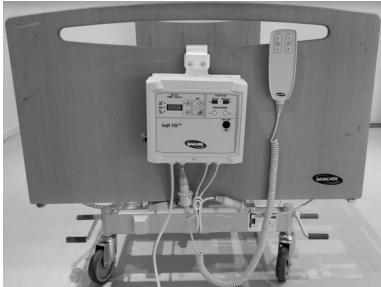
Collect the motor cables in a bundle and tighten it with a zip tie, move the bed up and down to make sure that the bundle is not clinging on any bed parts and moves freely.
