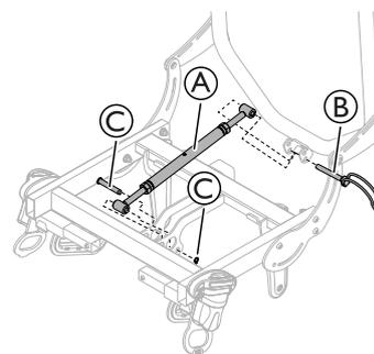
1. Attach the Rigging screw (A) in the front and the rear attachments.
