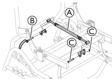
1. Attach the Rigging screw (A) in the front and the rear attachments.
