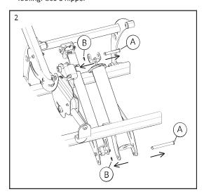
4. Remove the two safety pins (A) and locking washer (B) of the gas piston. Tooling: Use a nipper
