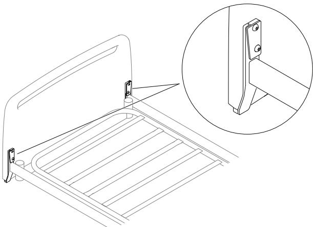
Press down firmly and ensure the bed end is fully seated on the brackets.
