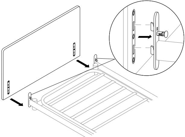
Align the slots in the bed end with the tabs on the Sanne bracket and place the bed end onto the tabs.
