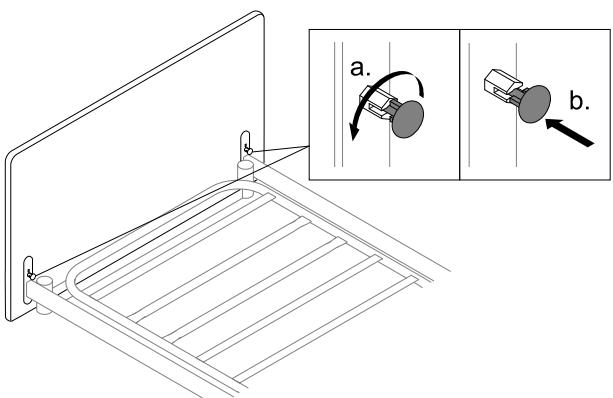
Rotate the locking pin and allow it to engage with the bed end on both sides.
