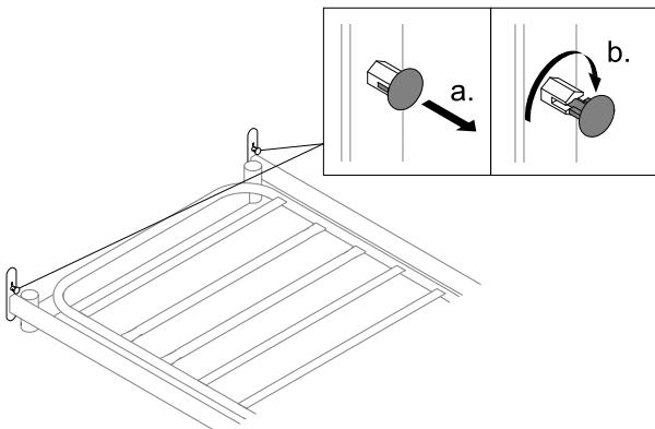
Pull out the locking pin and rotate by 90 degrees to disengage from the bed end on both sides.
