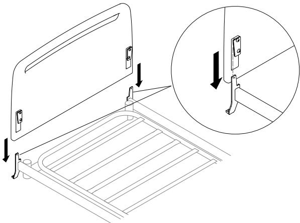
Align the slots on the bed end with the tabs on the Quick bracket and lower the bed end onto the brackets.
