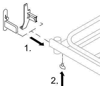
1. Insert the bed end brackets into the side tubes of the mattress support platform.
